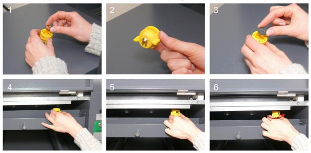
Prior to switching the machine on for the first time, one should check whether the protective cable is correctly connected. All containers (picture 1) should be controlled before starting operation. The container with pre-coating liquid should be shaken every day (picture 2). Connect the deposit tank. Cut the hose to the desired length. Do not bend the hose. Do not make a loop. Do not place the tank above the outlet.
